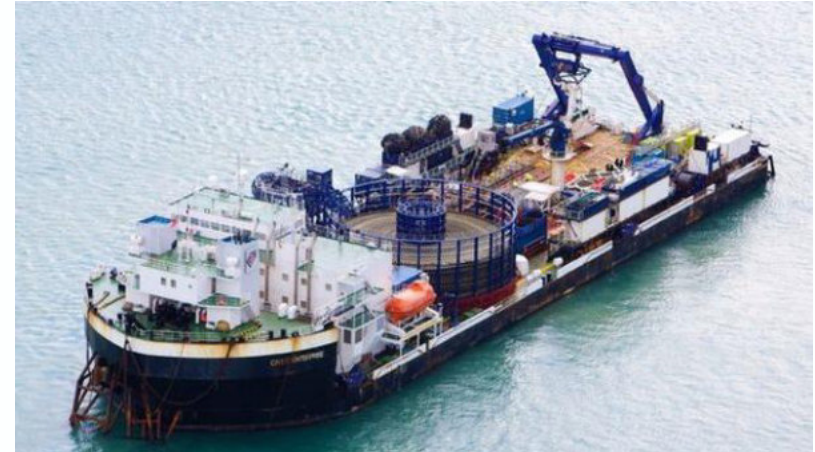
Cable lay barge Cable Enterprise
